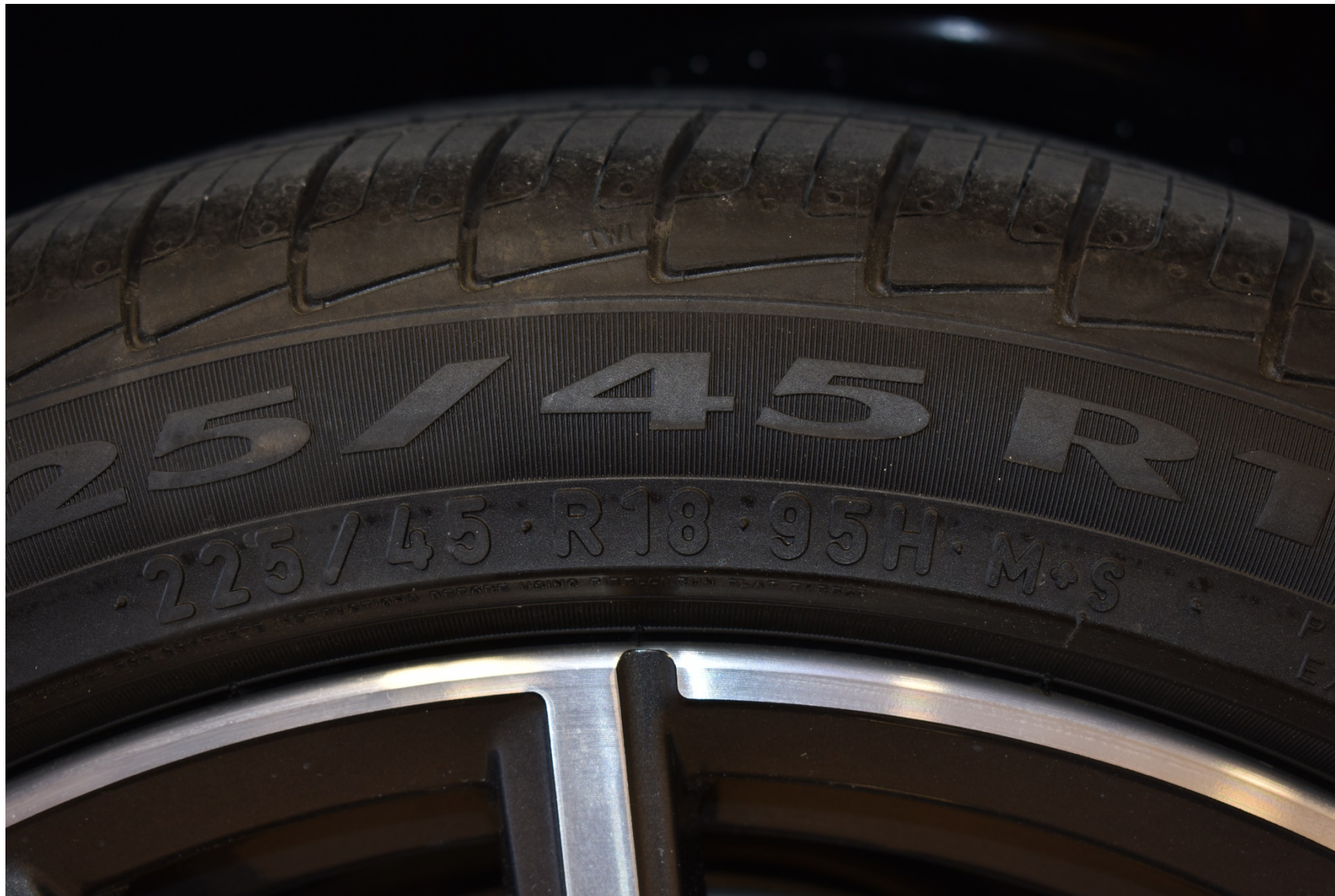
FIGURE 5.7 TIRE SHOWING SIZE, LOAD, & SPEED INDEX
